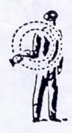
BACK - Swung vertically in a circle at half-arm's length at right angle to the track.
