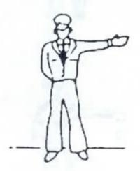
ASPECT: Raised and lowered vertically, in the direction of the Train Operator.
