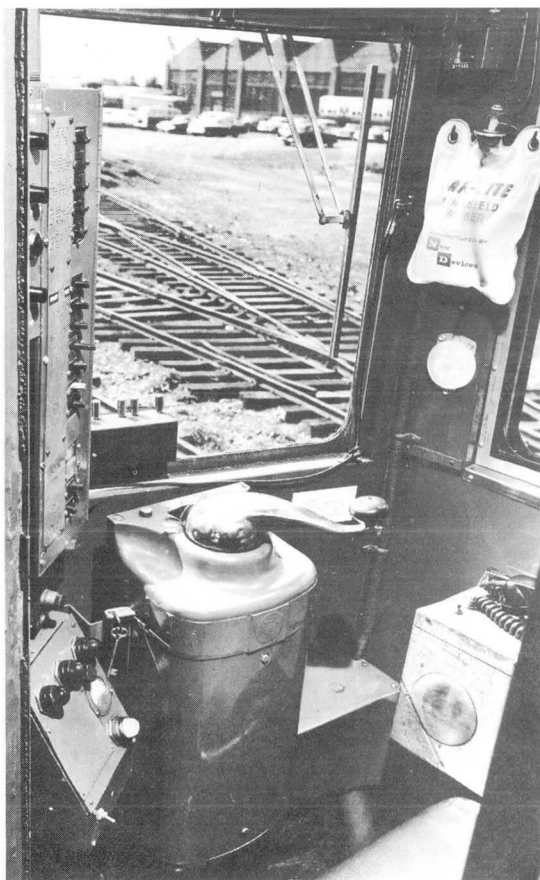
Car 51, one of two high-capacity cars assigned to Skokie Swift during the report period, is shown here after being refurbished and equipped for the high-speed service. The view at the left shows the operator's cab; note windshield washer and train telephone. Passengers may walk to any part of the car by passing through the diaphragm-enclosed archways which connect the three compartments (below). Each car has seats for 96 passengers.
