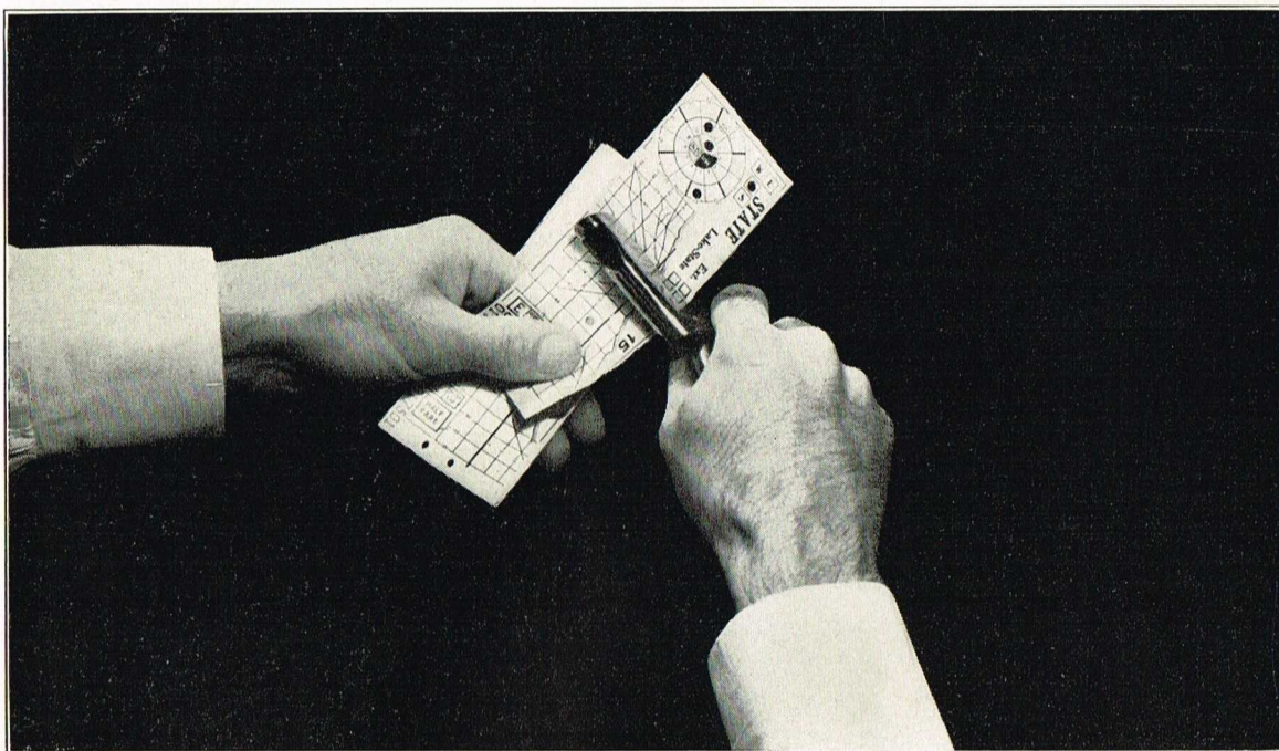
Proper method of holding punch (at right angles with the side of the transfer) when punch marking the line of zones between 3000 and 4500 west.
